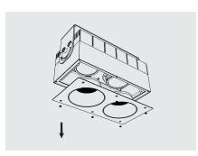
1. Unfasten front screws to detach front cover plate and reflectors.
