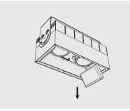
2. Disconnect cables attached to LED driver and unscrew bracket to remove LED driver for replacement.
